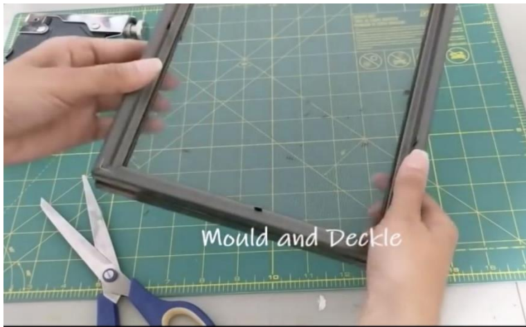
Trim the edge and place the second frame on top of the first, so that the front of both frames face each other.
