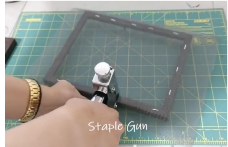
Pin or staple mesh to the front of one frame. (You can use an old pillow case or any fine material if you don't have mesh)
